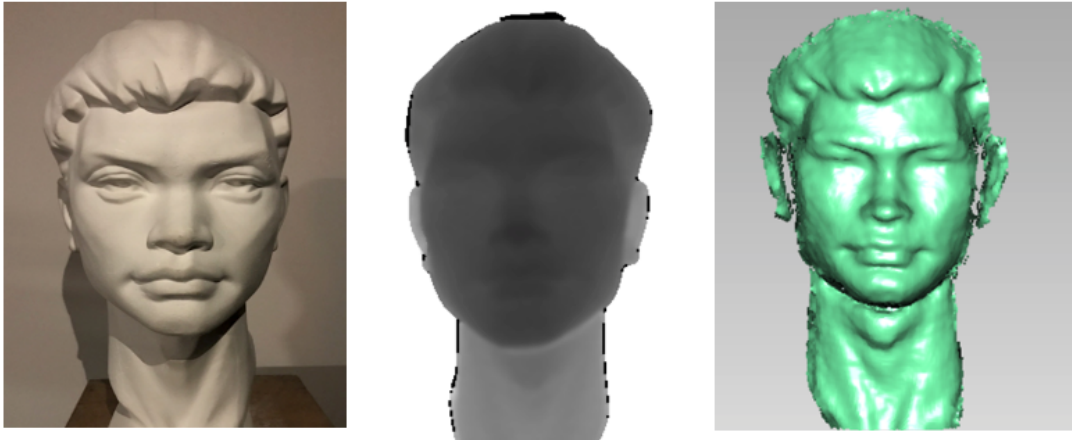
From left to right: original target, IR depth map, 3D point cloud generated from IR depth map
