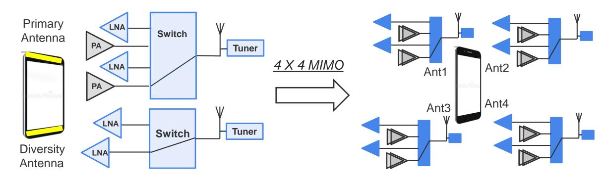
■ Technology: SiGe and RF SOI for LNA; RF SOI and in the future RF MEMS for antenna tuning
