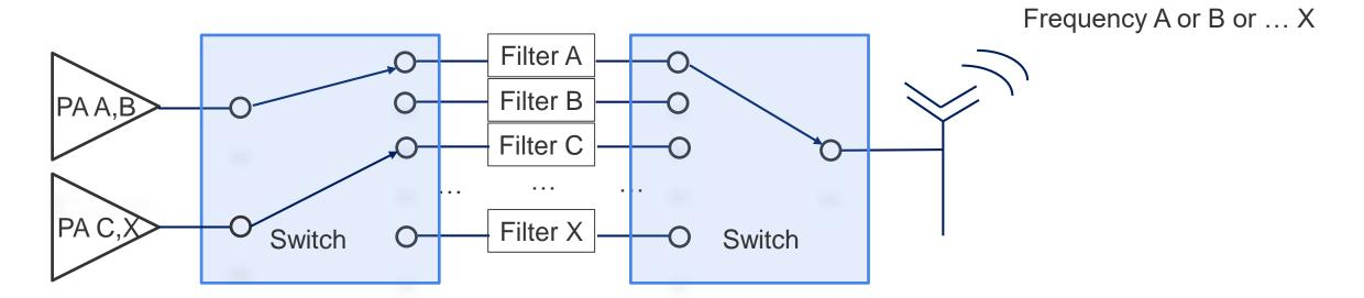
Technology: 5G RF switches in handsets are generally built in high-end RF SOI technology
